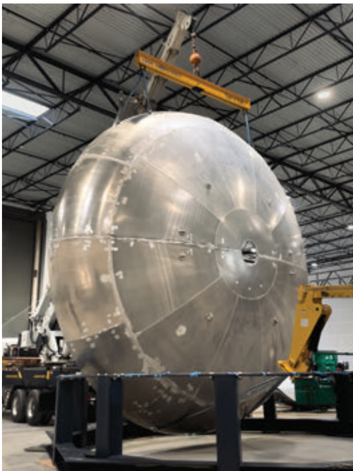
Flipping one of the 8 meter domes as part of the build process for the prototype StarMax hull.
